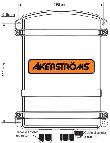
Mount the receiver upright with the cable glands facing down. The receiver shall be mounted on a flat surface with screws suitable for the surrounding environment. Note! If the plastic spacer is mounted the screws needs to be 20 mm longer.
